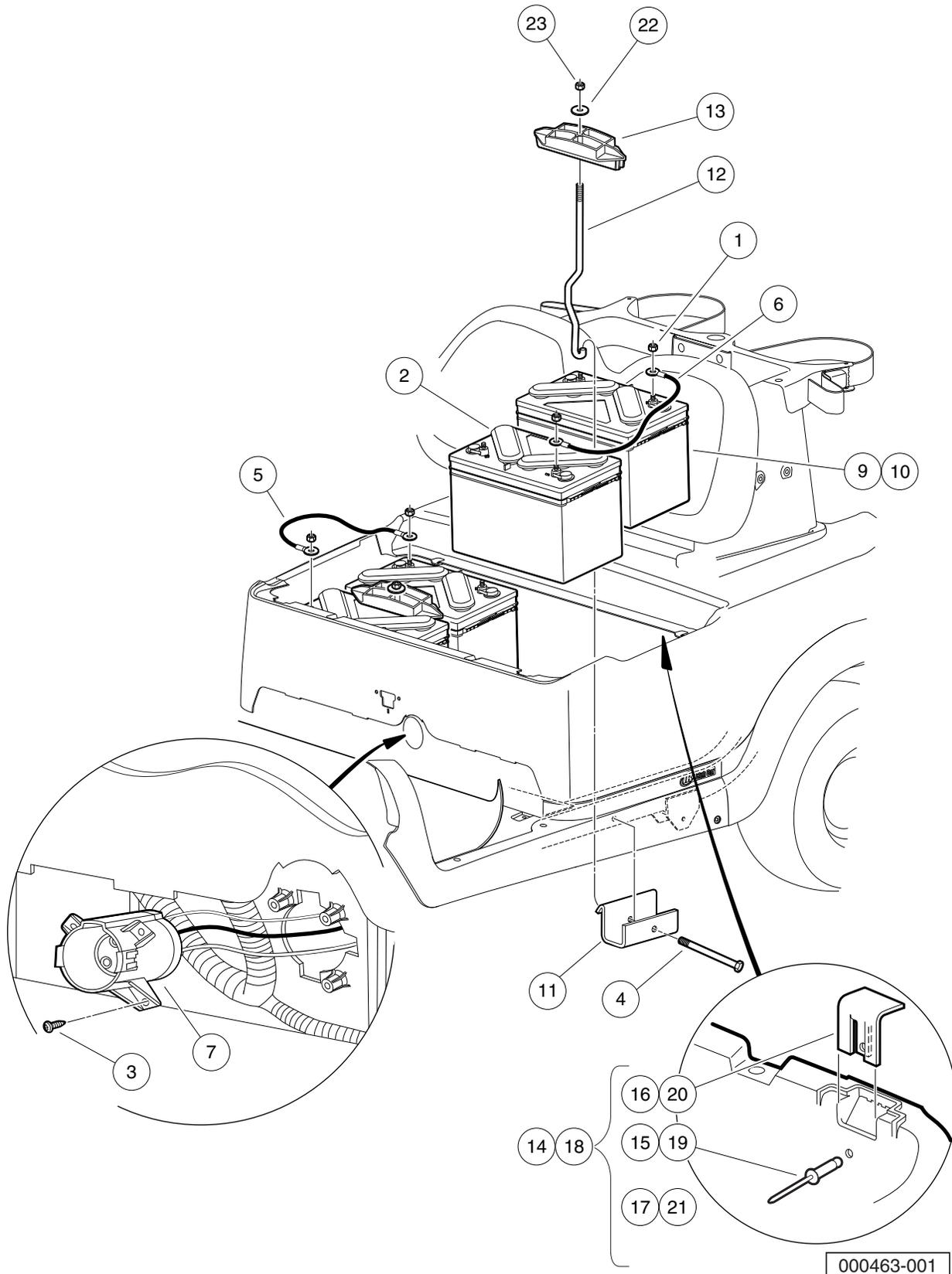
**BATTERIES, BUCKET, AND CHARGER RECEPTACLE - ELECTRIC VEHICLE**
