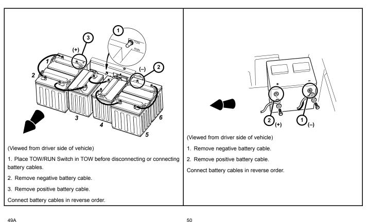
Figure 3 Battery Cable Removal – 6x8-Volt Battery Configuration
