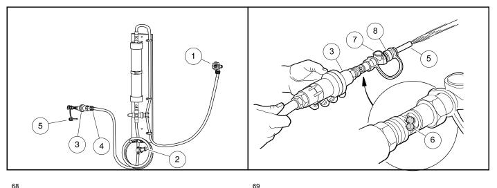
Figure 31 Connecting Hose with Filter to Water Source
