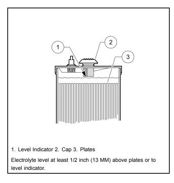
Figure 28 Battery Electrolyte Level
