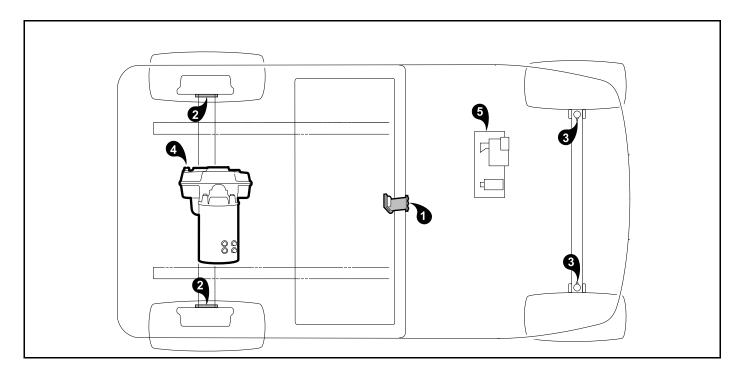
Figure 26 Lubrication Points – Electric Vehicles
