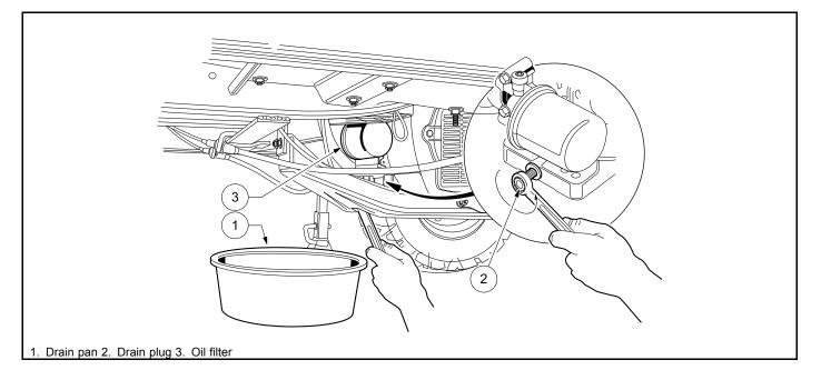
Figure 38 Engine Oil Drain Plug and Pan
